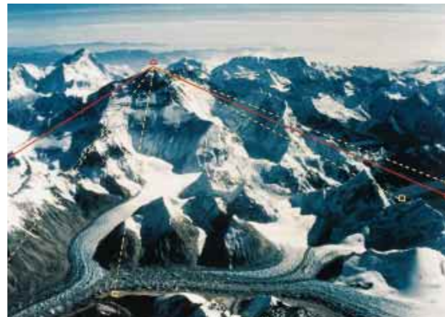
The beacon at the peak of Mt. Everest was targeted from six sites in Tibet (left) and Nepal (right).
