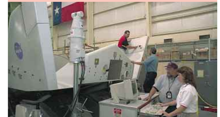
The Laser Tracker has been lifted up to get a wider working area.
