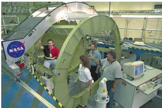
Part of the prototype X-38, a spacecraft model for the emergency crew return vehicle (CRV), the lifeboat for the International Space Station.
