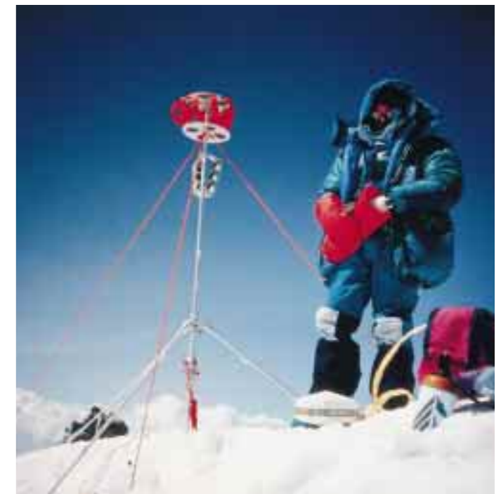
Right: Peak target and Leica GPS on Mt. Everest.
