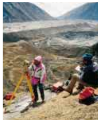
Leica T3000 theodolite and DI3000 distance meter in action in the Khumbu glacier valley (Nepal).
