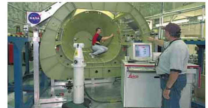
The reflector is moved along the inside wall for inspection.
