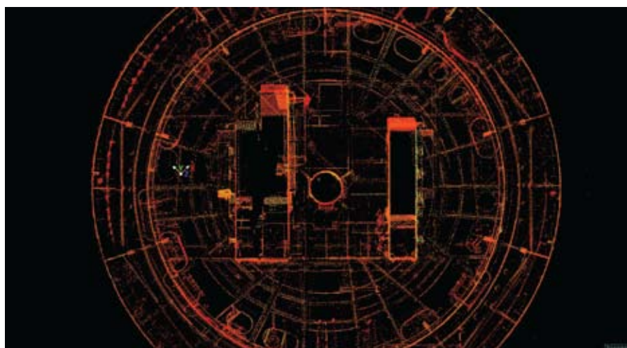
Above left: Scan team member Donald Axtell positions a Leica HDS 6000 laser scanner near a commemorative plaque on the surrender deck of the USS Missouri. Top: A point cloud of the USS Missouri’s port bow from below reveals a virtual snapshot of the historic naval vessel. Bottom: A plan view of the powder handling area in turret No. 2 displays a projectile storage area in the upper outer ring.
