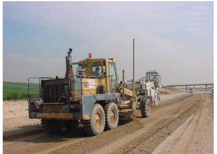
Leica Machine Control System for Graders on a Hanomag Grader with Wirtgen Recycler in front
