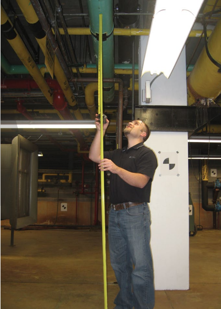
Field measurement requires measuring spaces by hand using a tape measure. Engineers with Sebesta Blomberg estimated that this method would provide good to marginal accuracy.
