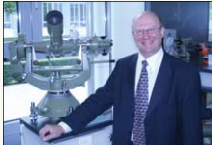
Leica Geosystems executive vice president Eugen A. Voit poses with a Wild T4 micrometer theodolite. Originally manufactured in the 1950s, it is the largest of the Wild theodolites.
