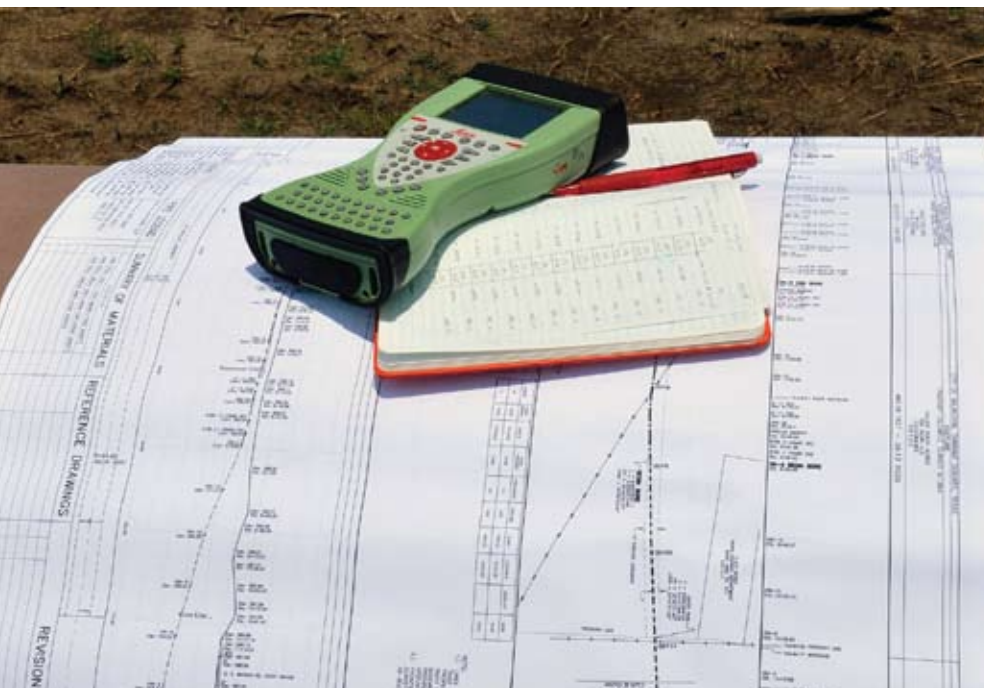
The survey crew double-checks the station data on an as-built pipeline against their Leica Viva Uno handhelds.
