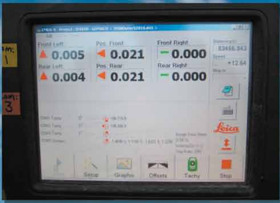
Leica LMGs Machine Software shows operator all phases of control from one easy to read screen.
