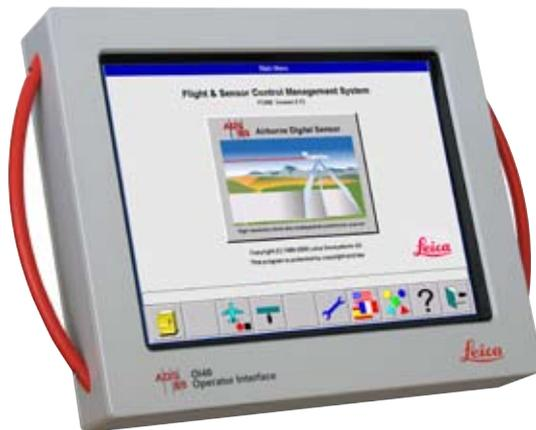
The Leica OI40 is a high-resolution pressure-sensitive LCD touch screen that operates the Leica ADS80 Airborne Digital Sensor.
