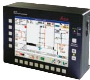
The Leica OC50 for the pilot is a rugged single-board computer with a high contrast LCD color screen designed for a cockpit environment.
